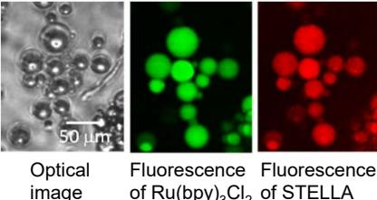
Biocompatible hydrogel oxygen sensor was fabricated.
