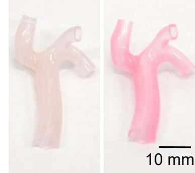
Over 47 μm PVA to protect from acetone
