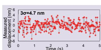
Measurement of reliability when the probe was fixed.
